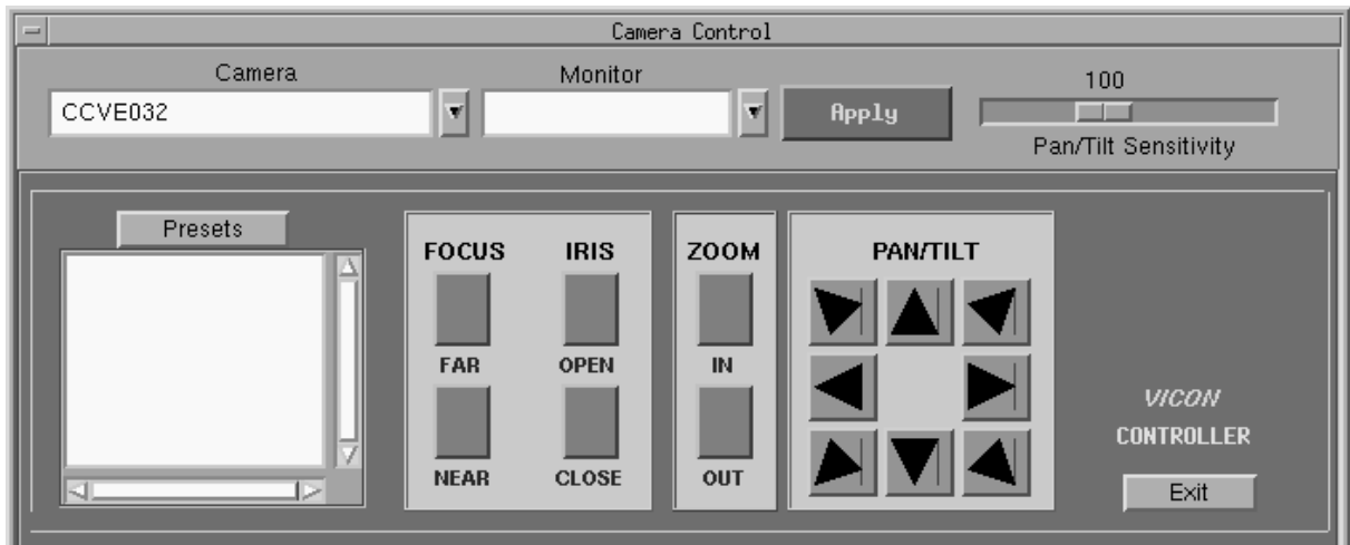
Figure D-5. Sample TMC Operator CCTV Camera Control Interface
