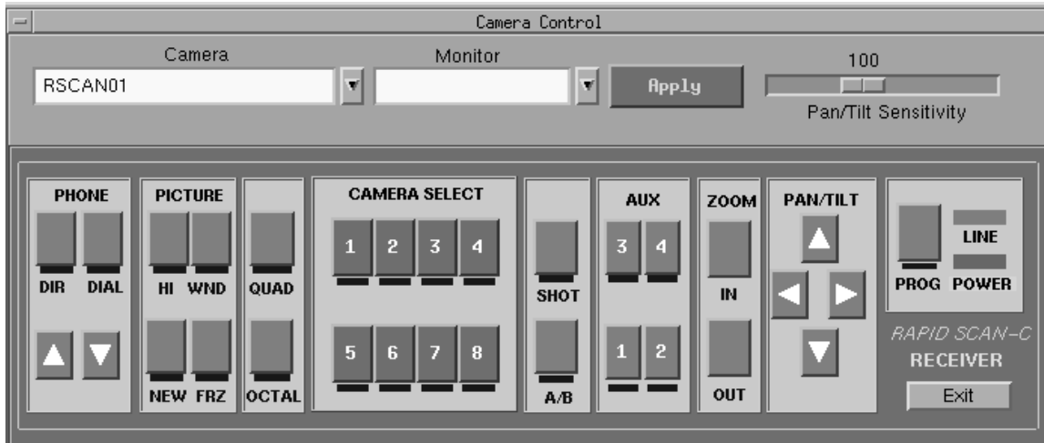
Figure D-6. Sample CCTV Interface for Cameras with Additional Capabilities
