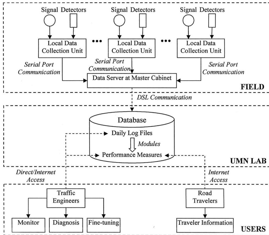
Figure 14 The SMART-SIGNAL System Architecture
